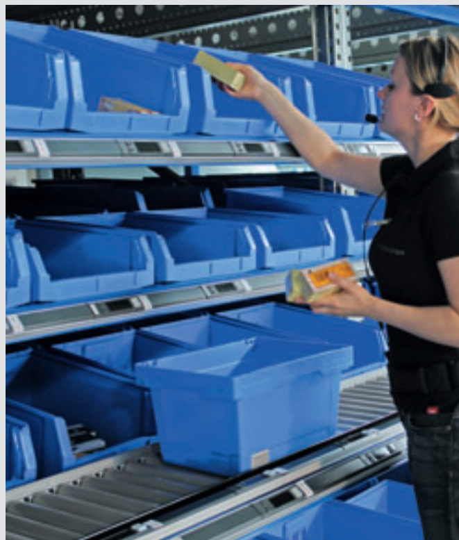
KDR with integrated conveyor system, pick-by-light and KMB returnable containers
