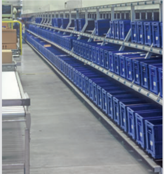
Flow beds combined with pick-by-light and FK boxes for order-picking
