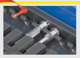
Vacuum-formed insert with precise positioning of turned parts
